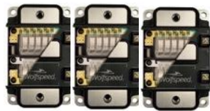
Lucid Traction Inverter with 3 10-die modules
