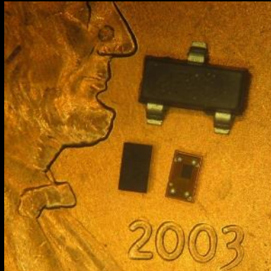
WL-CSP devices on a U.S penny. A SOT-23 device shown for comparison
