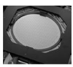
WaferPak<sup>TM</sup> Cartridges interface from the FOX-1 or FOX-15 system to the customer's wafer to be tested or burned-in. They contain micro-miniature probes to contact all of the die on a wafer in a single touchdown. WaferPak Cartridges are custom designed uniquely for each customer wafer application to interface to the unique pad positions of a wafer design. When used in a FOX system, WaferPak Cartridges enable the production of Known-Good Die (KGD) for use in multi-chip packages.
